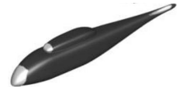
▲ Ice accretion shape with FENSAP-ICE**
